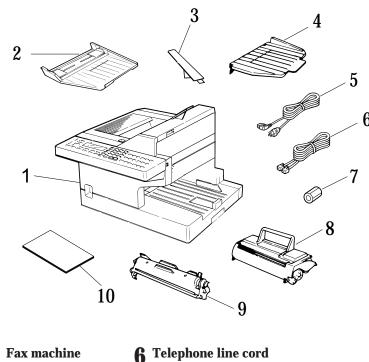
2Document hopper7Ferrite core3Paper hopper8Toner cartridge4Document tray9Drum cartridge5Ac power cord10Operating manual (this one)
